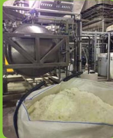
Increased chlorine input at high alternative fuels use rates requires a Bypass System to ensure a reliable kiln operation. A Bypass System drains a fraction of kiln gases along with calcined meal entering the kiln, which features a high concentration of salts and alkaline compounds that otherwise will create heavy buildups in the kiln and preheater. As part of this extracted material can be recycled into the production process, excess dust needs to be disposed.
