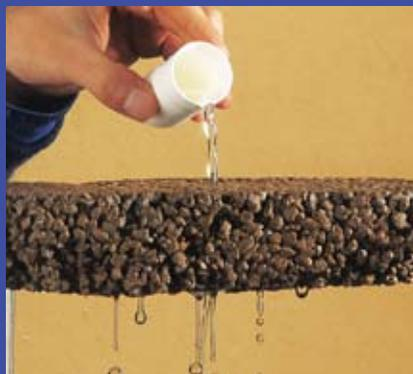
**Permeable concrete** that allows rainwater to filter through, reducing both heat build-up and flood risk.
