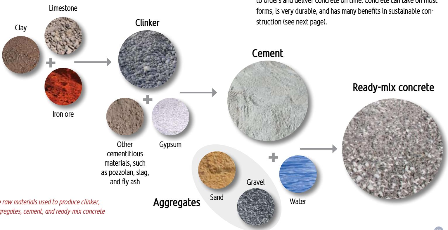
*The raw materials used to produce clinker, aggregates, cement, and ready-mix concrete*
